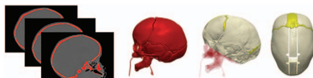
FIGURE 7. Creation of FE model for modeling of spring cranioplasty; segmentation of CT images (left); creation of a 3D skull model (center-left); identification of the region of interest for the modeling (center-right); reproduction of surgical osteotomies (right).
