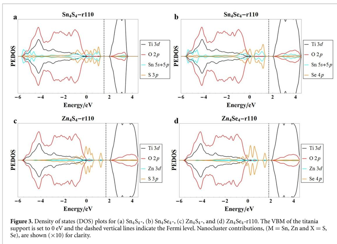
modification, Sn-derived states emerge in the energy gap. These states are due to the lone pair, as has been discussed in previous work on Sn chalcogenides [66, 67].
