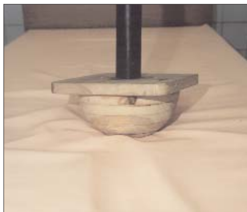
Fig 1. The wooden hemisphere indenter, prior to loading a replacement mattress
