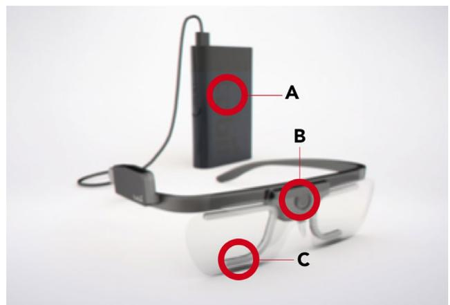
**FIGURE 2** The eye tracking glasses which were used to record participants. These are the Tobii Glasses 2 wearable eye tracker. (A) Recording storage, (B) scene HD camera, (C) infrared cameras (Tobii Technology / CC BY (<https://creativecommons.org/licenses/by/3.0>))
