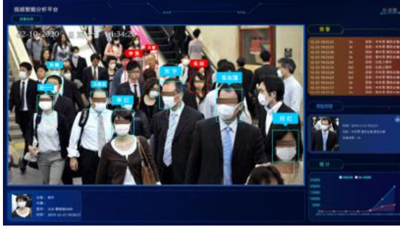
Fig. 2. The SenseTime's system can help to flag people who are not wearing facial masks automatically for building access control using artificial intelligence's facial recognition [3].
