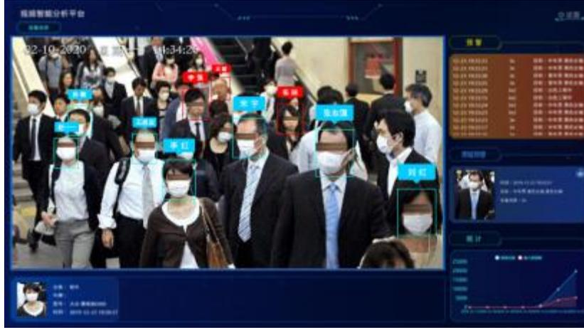
**Fig. 2.** The SenseTime's system can help to flag people who are not wearing facial masks automatically for building access control using artificial intelligence's facial recognition [3].
