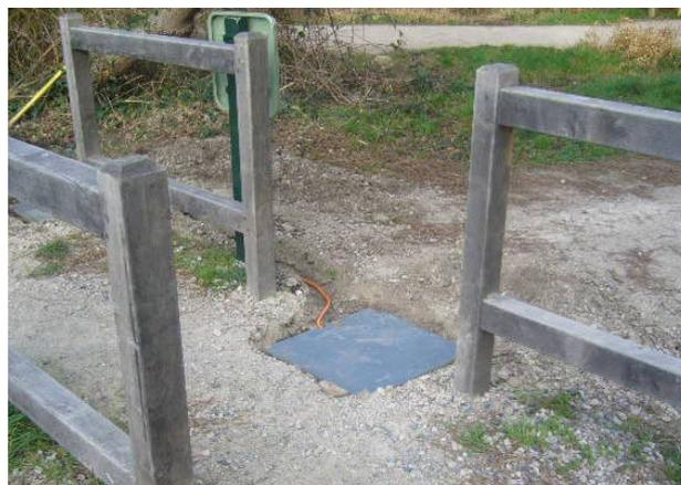
**Figure 7.** Eco Counter ‘SLAB’ installed at a pedestrian pinch point.
