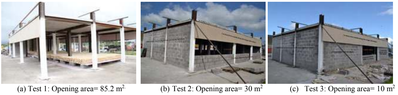
Figure 2 Different opening layouts were used for the three tests.
