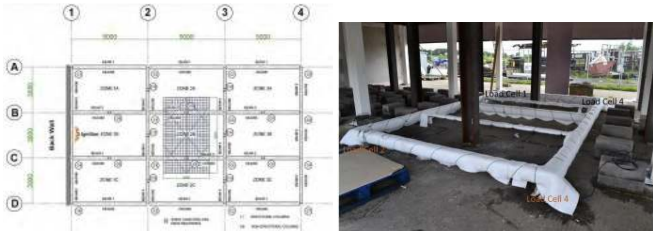
Figure 6. Position and arrangement of the mass loss recording through four load cells
