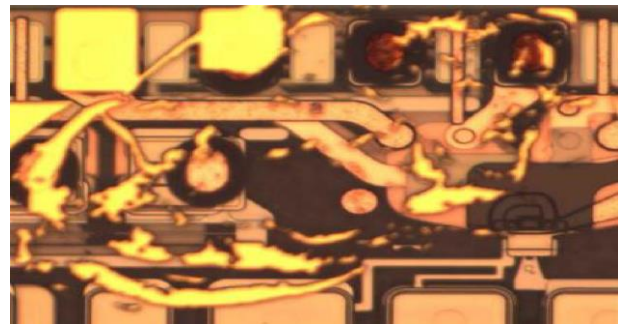
(a) Gold resist in various stages of damage
