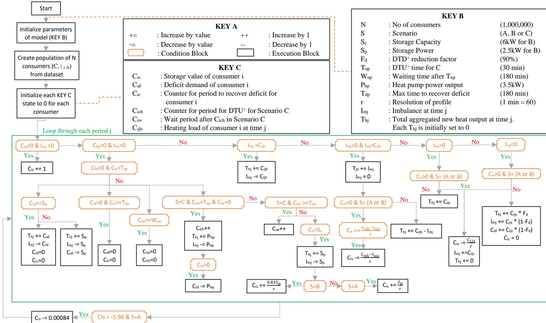
**Figure 3.** Flowchart of DTU<sup>+</sup> and DTD<sup>+</sup> Simulation Model
