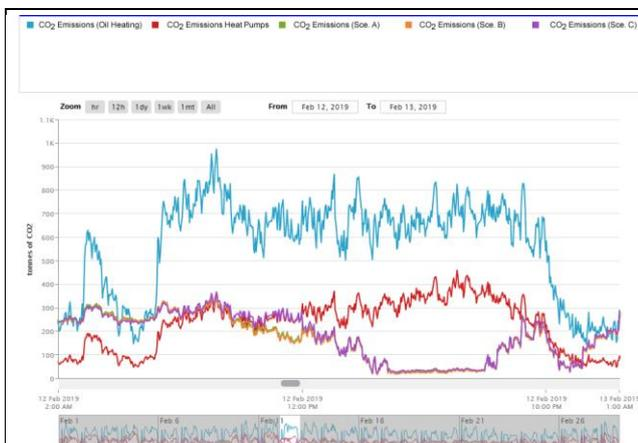
**Figure 8.** CO<sub>2</sub> Emissions of Oil heating vs Heat pumps in normal operation vs Heat pumps in the three Scenarios
