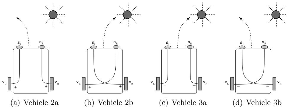
Figure 1: Schematics of Braitenberg Vehicles 2 and 3
