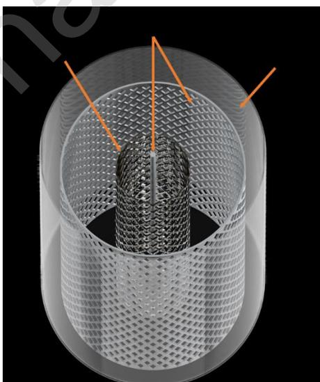
Figure 3 ± Electrode configuration for anodisation
