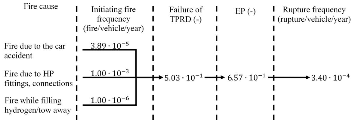
Figure 4. Frequency of a tank rupture in a localised fire.
