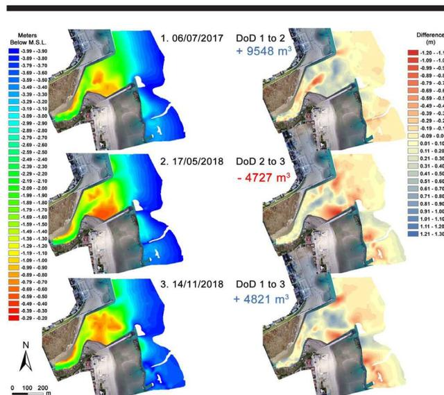
Figure 2. DEMs and DoDs of bathymetric surveys of the Savio river outlet. To note that the dates in the figure are in the format dd/mm/yyyy.
