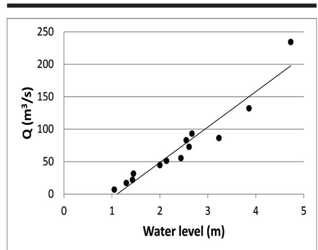
Figure 3. Relationship between measured river water levels (referred to MSL) and measured discharge values ( $Q$ ).
