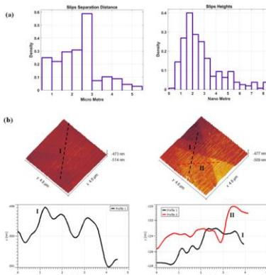
**Fig. 4.** Shows a) probability distribution map of slips separation distance and height after 1000 cycles. HS-AFM topographic maps of the surface inside two different grains after 1000 cycles. The arrows indicate the trace of the slip planes: b) different orientations. The profiles I, II taken along the lines I and II respectively show steps. The lines are started from left to right.
