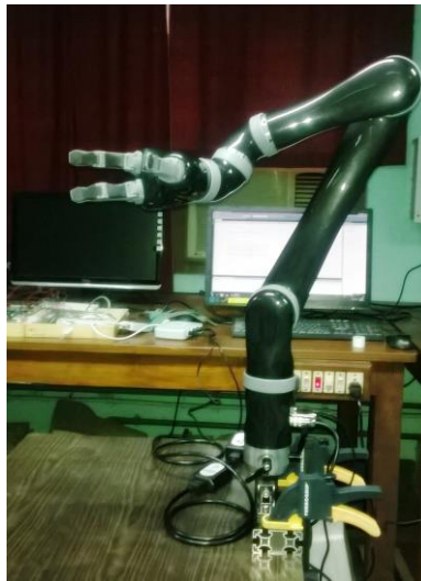
Fig. 2. Jaco Robot Arm setup in our lab
