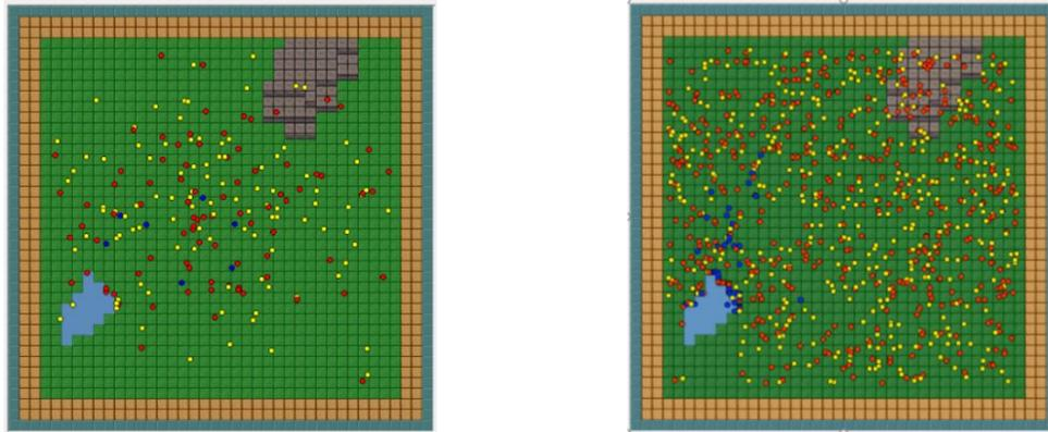
**Figure 2. Simulation with Centralised Message Board component. A swarm of red and yellow robots was tasked with finding water and recruiting other robots to help analyse it. Robots change colour to blue when responding.**
