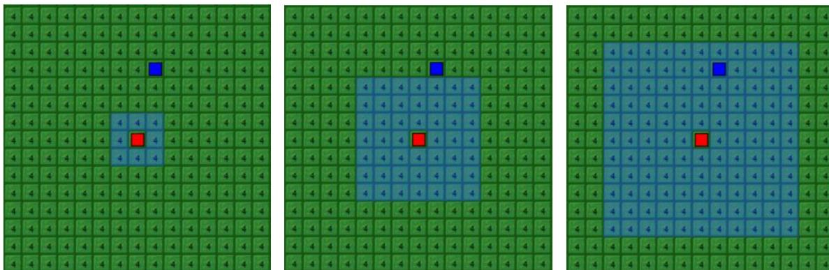
**Figure 6.** The blue area surrounding the red robot depicts the range of the signal strength. (a) Signal strength is set to 1 level, this covers the cells immediately surrounding the red robot. (b) When the signal is set to 3 the range is 48 cells and 3 levels around the robot. (c) A Signal of 5 has a reach of 120 cells, in this scenario the blue robot would be in range to receive a help message from the red robot.
