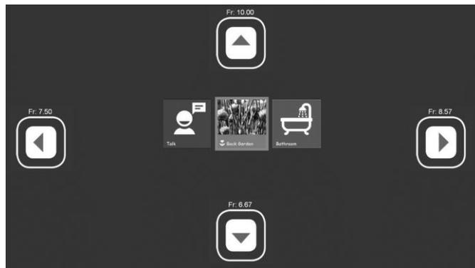
Fig. 1. The Visual Interface Application with on-screen stimuli located at the edges of the display. Each stimulus flickers using unique frequencies (left:7.5 Hz, up:10 Hz, right:8.57 Hz, down:6.67 Hz).
