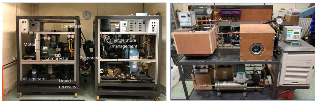
Figure 1 Test rig used for lubricant analysis at Ulster University: HTHP (left), viscosity measurement (right)
