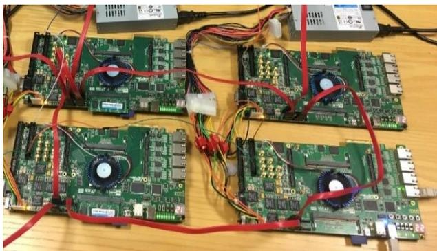
Fig. 5. A 4 FPGA AstroByte platform with SATA connections
