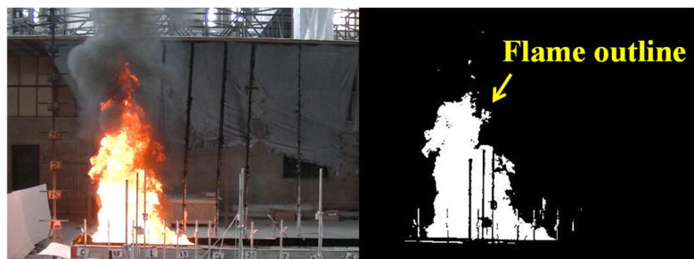
Fig. 4. A schematic diagram of the flame processing method ( R>200, G>100, B>50 )
