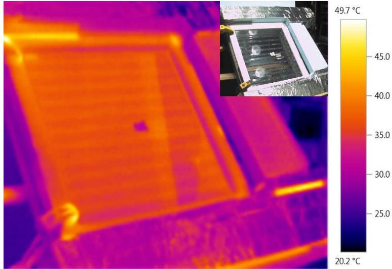
Figure 7. IR image showing temperature distribution on the surface of the CoPVTG prototype with Illumination incident at 20° (data from 15:35:  $T_i=34.3^\circ\text{C}$ ,  $T_o=35.7^\circ\text{C}$  and  $T_a=25.7^\circ\text{C}$ ).
