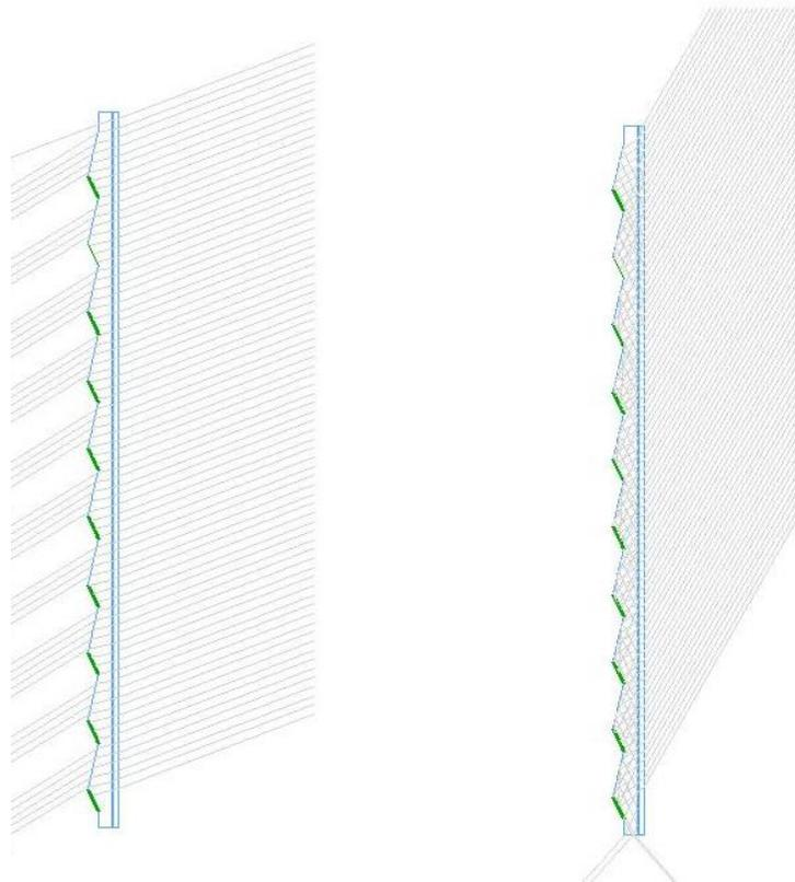
Fig. 2. Ray trace diagrams demonstrating the control of beam solar radiation transmittance by TIR at the concentrating lens. Light incident at  $20^\circ$  (left) and  $55^\circ$  (right) from the perpendicular to the surface of the glazing.
