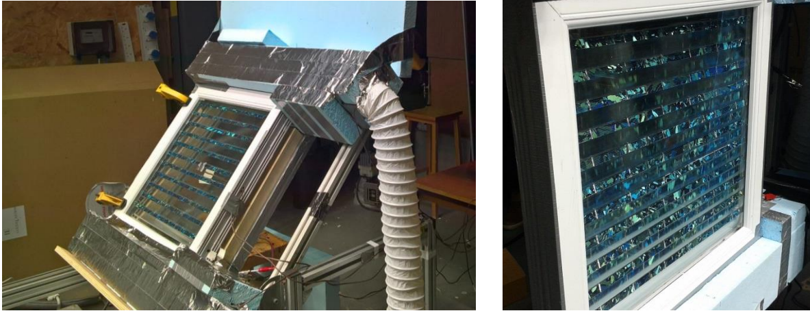
Figure 4. The experimental CoPVTG prototype (left) and a demonstration of TIR at the concentrating lens (right).
