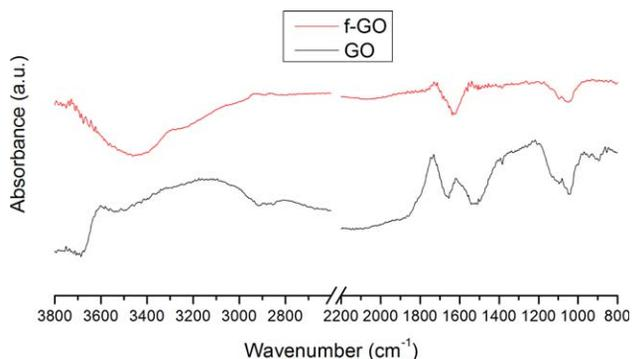
FIG. 2. FTIR absorbance spectra showing GO (bottom) and f-GO (top). [Color figure can be viewed in the online issue, which is available at [wileyonlinelibrary.com](http://wileyonlinelibrary.com).]
