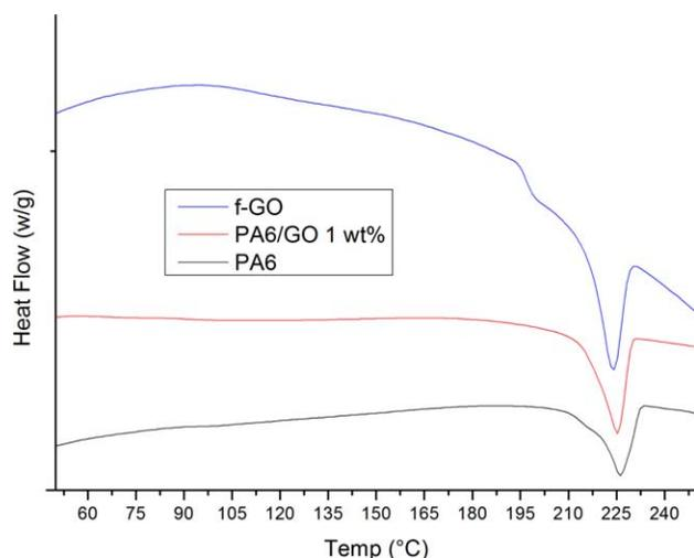
FIG. 8. DSC exothermic curve for neat PA6, PA6/GO 1 wt%, and f-GO. [Color figure can be viewed in the online issue, which is available at [wileyonlinelibrary.com](http://wileyonlinelibrary.com).]
