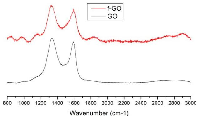
FIG. 3. Raman spectra of GO (bottom) and f-GO (top). [Color figure can be viewed in the online issue, which is available at [wileyonlinelibrary.com](http://wileyonlinelibrary.com).]
