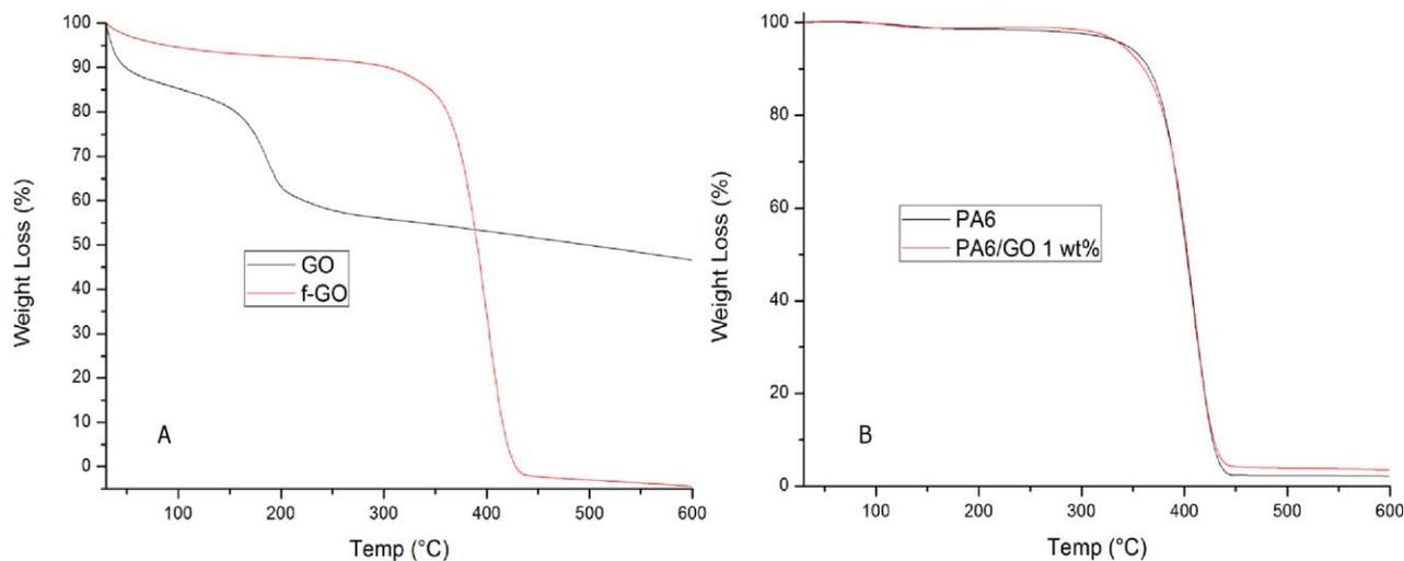
FIG. 7. TGA weight loss curves for (A) GO and f-GO and (B) neat PA6 and PA6/GO 1 wt%. [Color figure can be viewed in the online issue, which is available at [wileyonlinelibrary.com](http://wileyonlinelibrary.com).]
