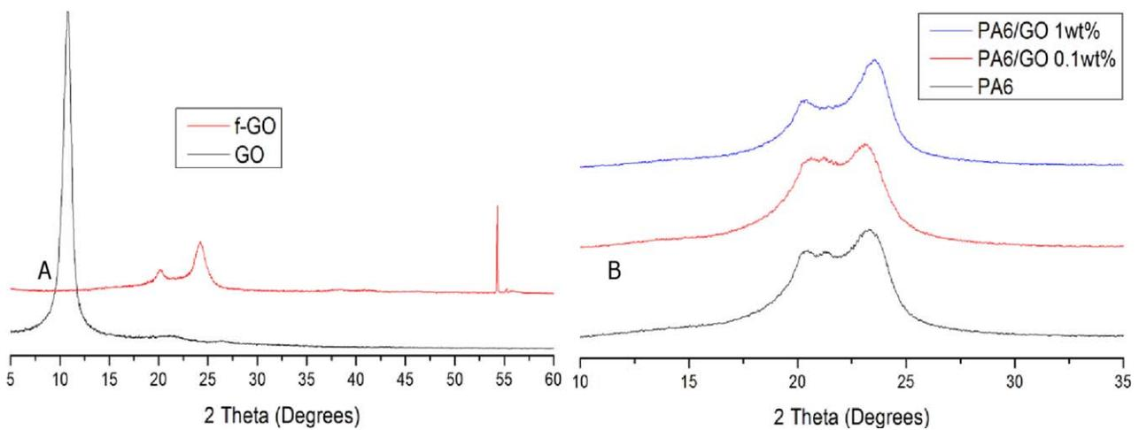
FIG. 5. XRD pattern of (A) GO and f-GO and (B) in ascending order PA6, PA6/GO 0.1wt% and PA6/GO 1wt%. [Color figure can be viewed in the online issue, which is available at [wileyonlinelibrary.com](http://wileyonlinelibrary.com).]
