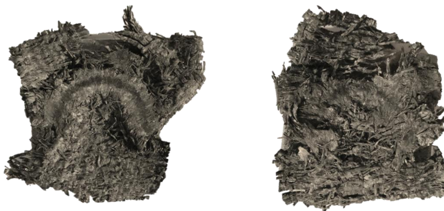
Figure 8: Final dynamic crush geometry in CF-UN-DYN (left) and CF-TG-DYN (right) specimens.
