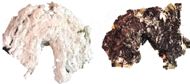
Figure 4: Final quasi-static crush geometry in glass GF-BA (left) and carbon CF-BA (right) samples.
