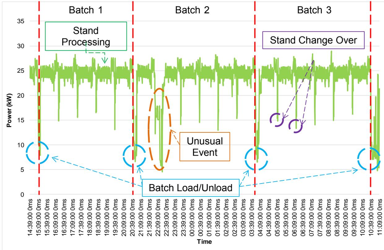
**Figure 3 GRND01- Power logged while manufacturing 3 batches**
