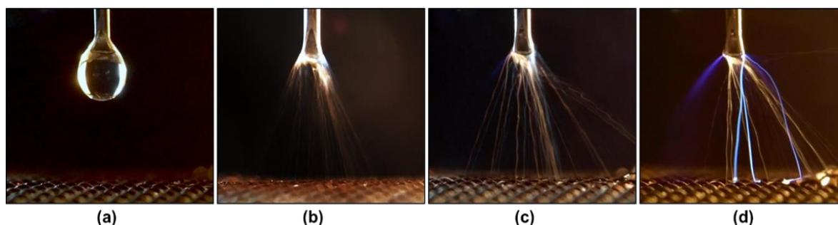
**Figure 2.** Photographs of the electro spraying of water in an 8-mm gap, water flow rate 0.5 mL min<sup>-1</sup>: (a) droplet without a high voltage, (b) electro spray with a high voltage applied, 5.5 kV, (c) electro spray combined with streamer corona, 6.5 kV, (d) electro spray with transition streamer corona-transient spark, 7.8 kV. Reproduced from Machala et al. [55]. All rights reserved.
