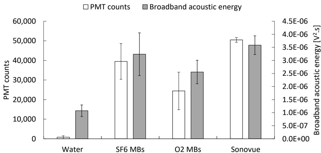
**Figure 2.** Sonoluminescence and broadband acoustic emissions produced by phospholipid-coated microbubbles driven at 1 MHz with an intensity of 3.5 W/cm<sup>2</sup>, 30% duty cycle, and 100 Hz pulse repetition frequency for 2 minutes. The total PMT (photomultiplier tube) counts above 6 mV in amplitude and broadband energy of acoustic emissions for three microbubble formulations and a water control are displayed. (n=3 runs of 1000 acquisitions each, error bars indicate standard deviations).
