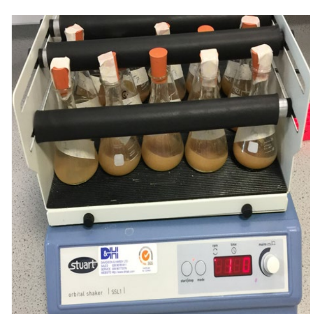
Triplicate samples on orbital shaker
