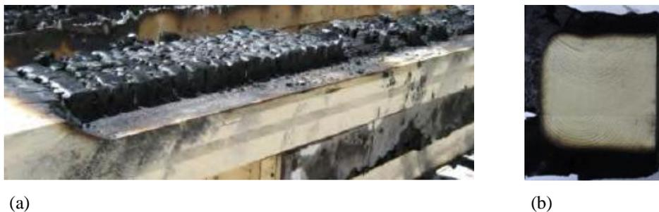
Fig. 2. Charcoal protective layer of (a) CLT panel [2] and (b) solid timber beam [5].
