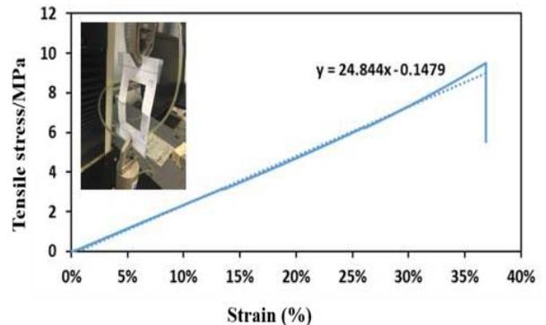
Fig. 3. Tensile strength test of PEGDA sample coated with parylene
