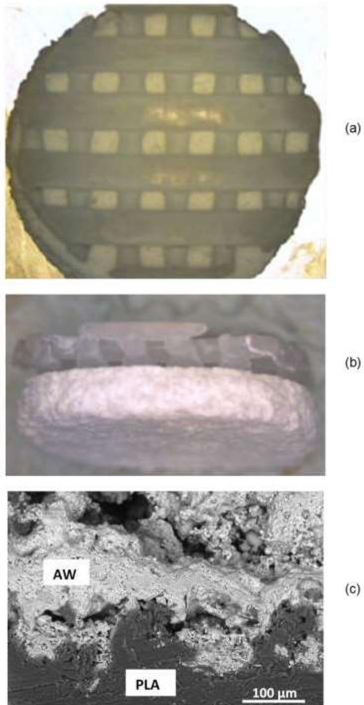
Figure 3. Images of bonded PLA/AW composite disks: (a) & (b) stereomicroscope images of 8 mm diameter composite disk, (c) SEM image of interface.
