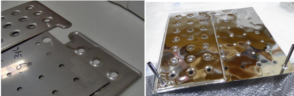
Figure 3. (a) Laser-cut sheets prior to welding, (b) Absorber after leak testing and electro-polishing, prior to black chrome plating.
