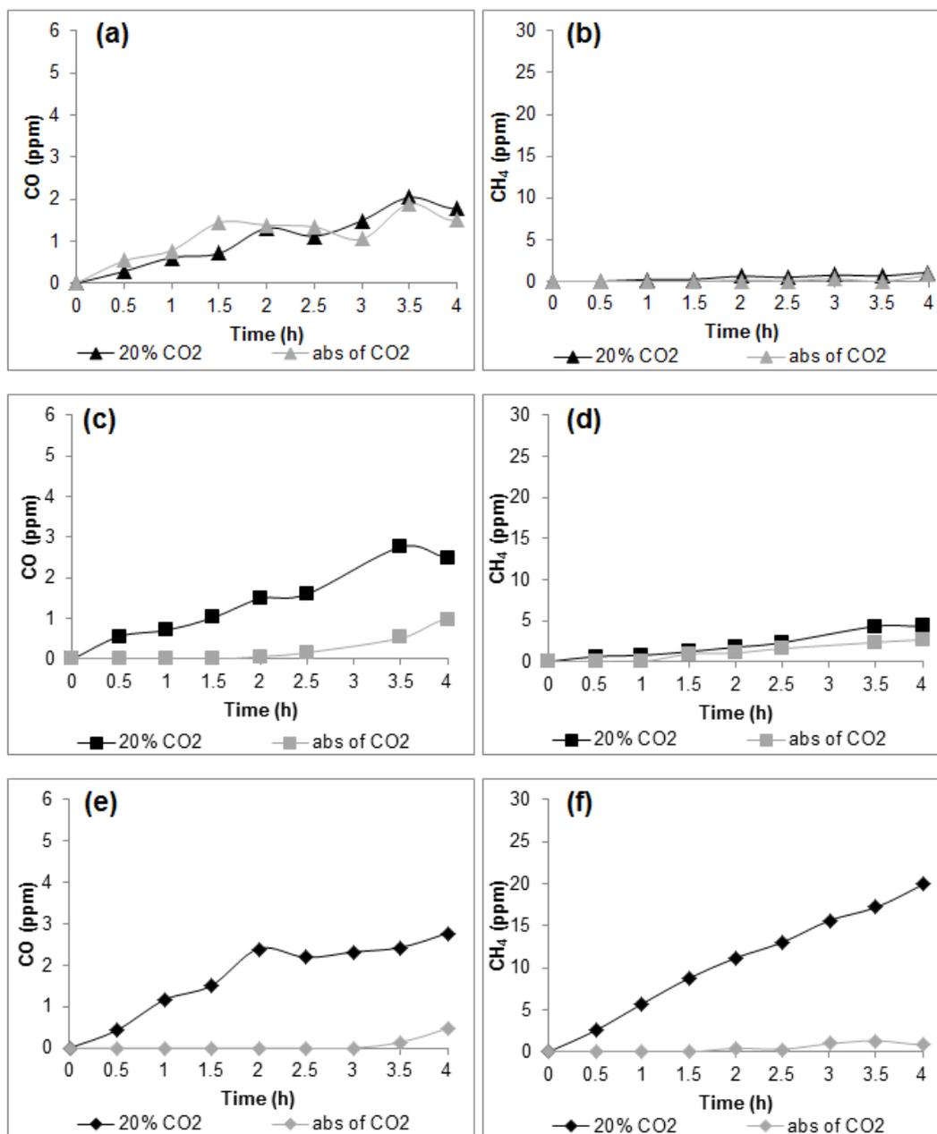
**Fig. 2.** CO and CH<sub>4</sub> production (in ppm) over time using different catalysts in the presence and absence of CO<sub>2</sub>. (a-b) TiO<sub>2</sub> (P25), (c-d) Cu-TiO<sub>2</sub>, (e-f) NT
