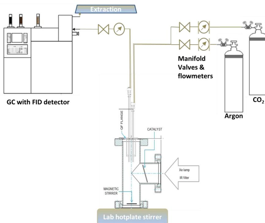
**Fig. 1.** Schematic diagram of the photocatalytic reaction apparatus
