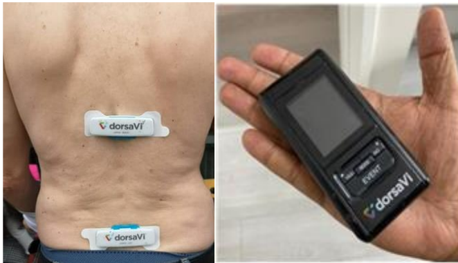
Fig. 1. (a) Sensor positioning using a fitting template, (b) RFD device for ViMove IMU sensors.
