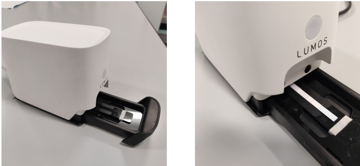
Figure 2. Lumos Reader device for capturing LFA images.
