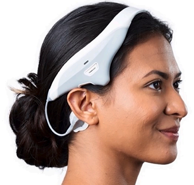
Fig. 2. The Modius Sleep device as intended to be worn, with electrode pads over the mastoid processes. Modius Sleep and sham devices had this identical appearance.
