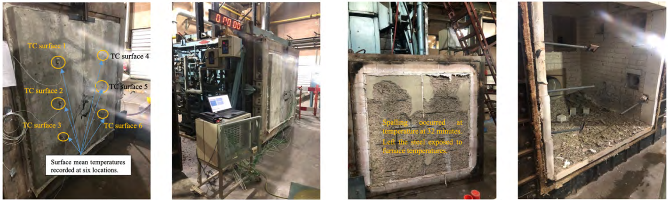
Figure 1. Precast sandwich Panel tested at Ulster University using ISO834 for 1 hour fire resistance
