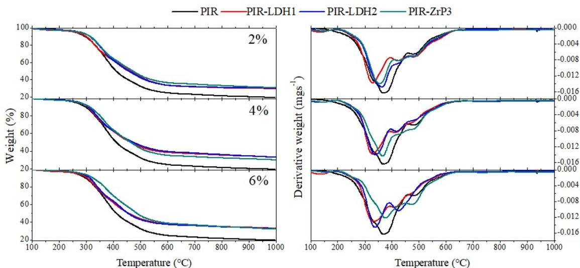
Fig. 2. TG (left) and DTG (right) of pure PIR, PIR-LDH1, PIR-LDH2 and PIR-ZrP3 in N<sub>2</sub> atmosphere.
