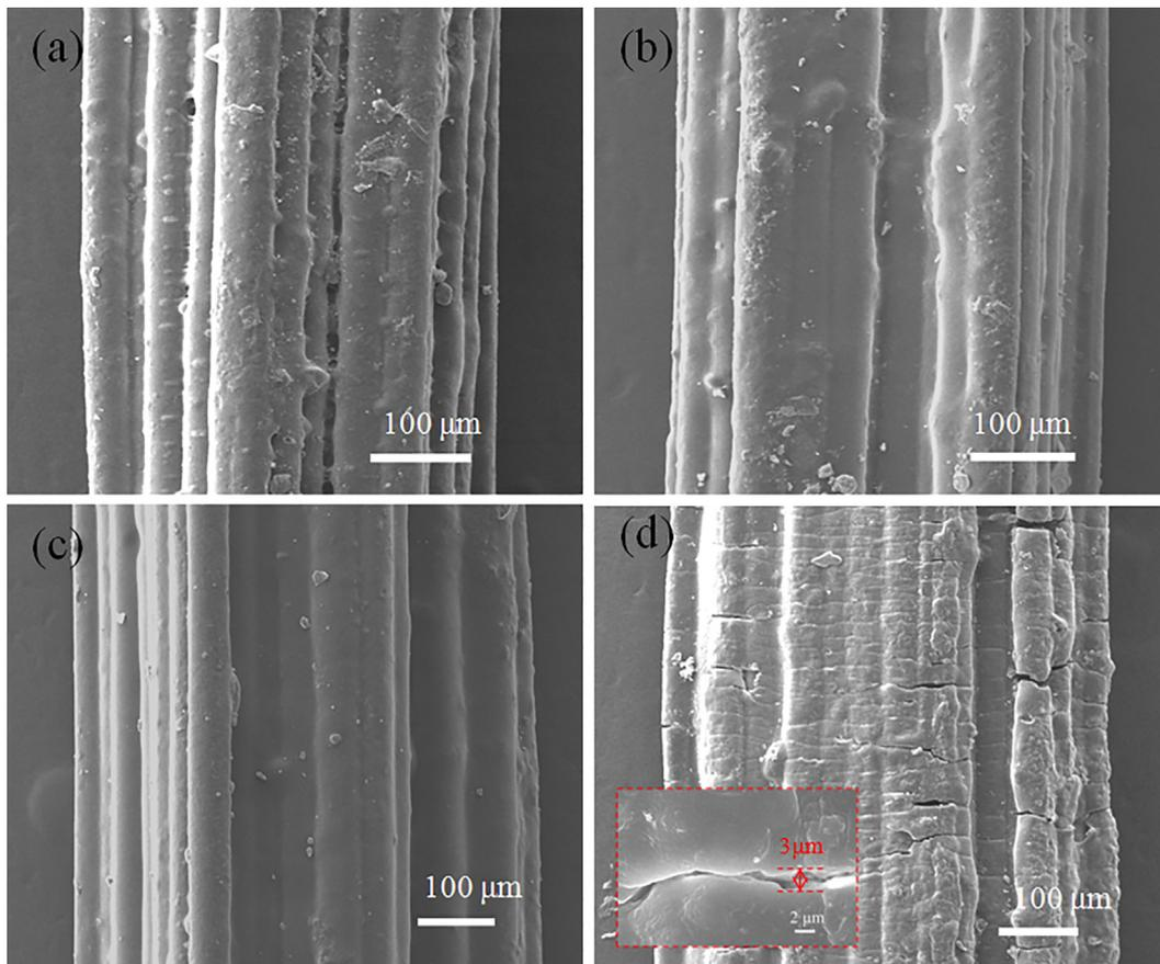
Fig. 12. SEM images of the UV treated fiber sensors ( $N = 3$ ) before and after a 30% cyclic strain: exposed to UV-light for (a) one and (b) two weeks; (c) after 2000 cycles for the sensor without UV treatment, (d) after 100 cycles for the sensor exposed to UV-light for two weeks.
