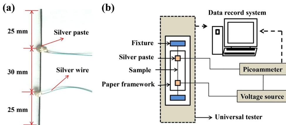
Fig. 2. (a) sample for strain sensing test and (b) schematic for strain sensing test.
