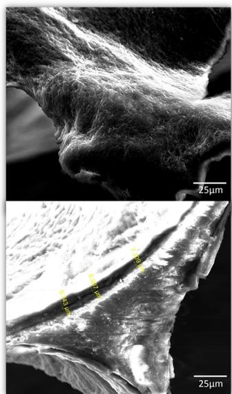
Figure 3: Film Surface (Top) Film Thickness (Bottom)
