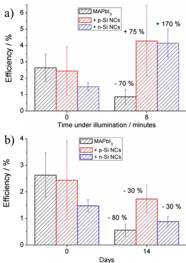
**Fig. 9.** a) PCE of MAPbI<sub>3</sub>, MAPbI<sub>3</sub> + p-Si NC and MAPbI<sub>3</sub> + n-Si NC devices at 0 min and 8 min illumination b) PCE of devices at 0 day and after 14 days in atmosphere.
