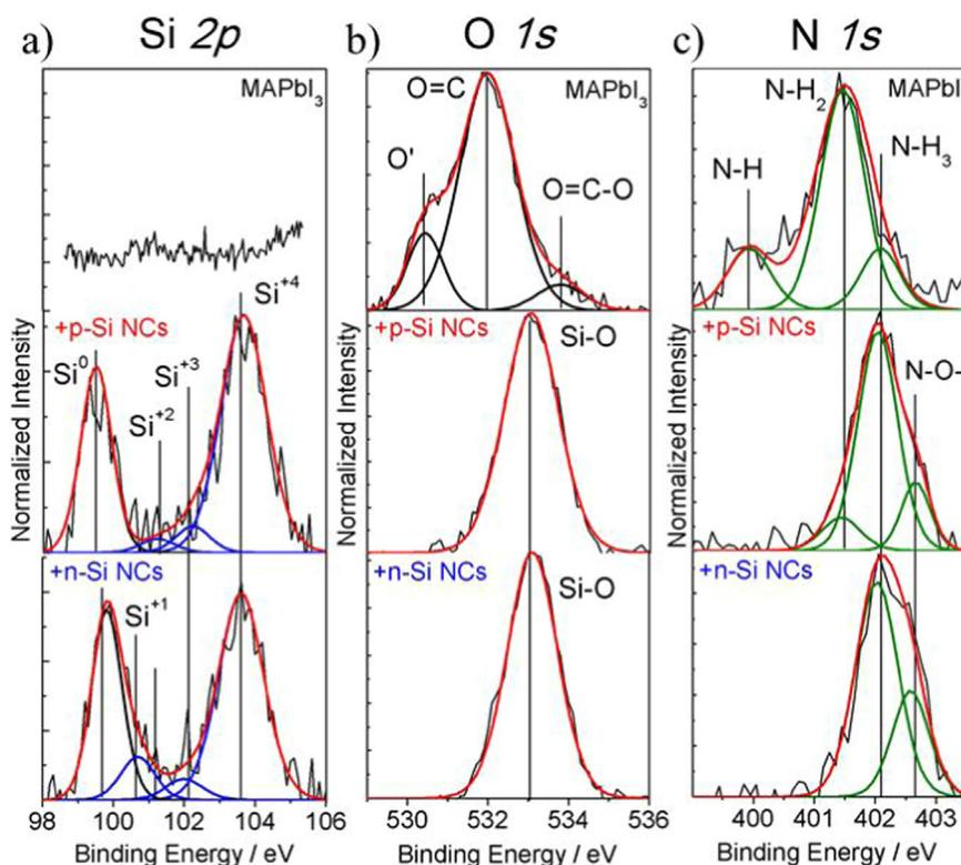
Fig. 2. X-ray photoelectron spectroscopy core level scans a) Si 2p b) O 1s and c) N 1s for spray deposited MAPbI<sub>3</sub>, MAPbI<sub>3</sub> + p-Si NCs and MAPbI<sub>3</sub> + n-Si NCs.
