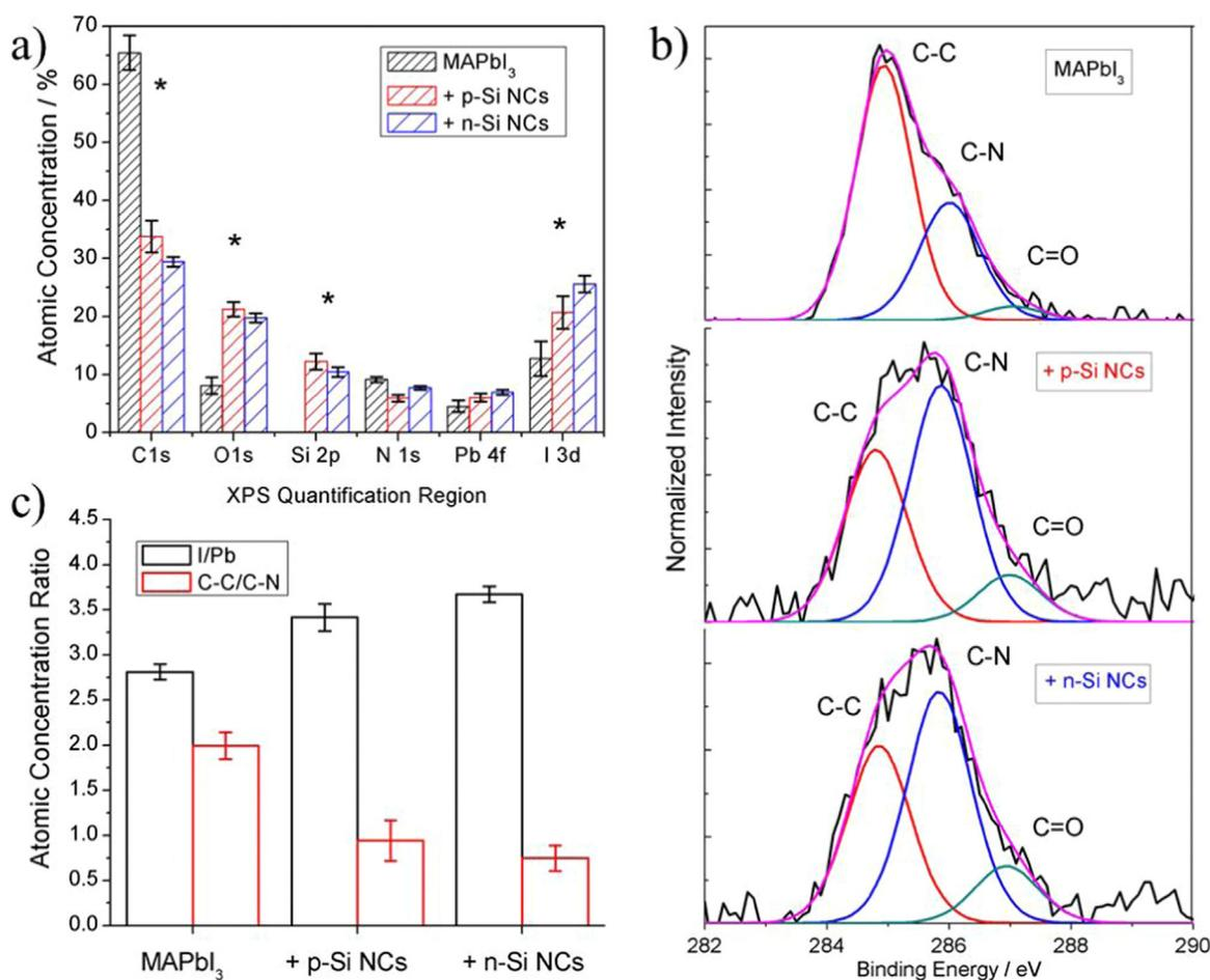
**Fig. 1.** a) Atomic concentrations for MAPbI<sub>3</sub>, MAPbI<sub>3</sub> + p-Si NCs and MAPbI<sub>3</sub> + n-Si NCs films determined from XPS measurements with b) C 1s region scans and c) changes in I/Pb and C-C/C-N atomic concentrations.
