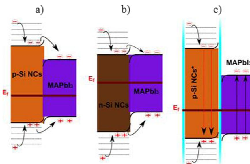
Fig. 7. Equilibrated energy band diagram of a) MAPbI<sub>3</sub> + p-Si NCs b) MAPbI<sub>3</sub> + n-Si NCs and c) MAPbI<sub>3</sub> + surface oxidized p-Si NCs\*.
