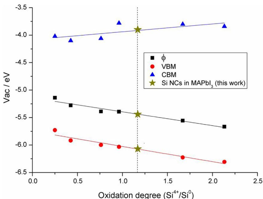
Fig. 6. Measured Fermi, VBM and CBM energy levels for p-Si NCs vs. p-Si NC oxidation degree expressed in terms of the ratio between XPS Si<sup>0</sup> and Si<sup>4+</sup> peaks.
