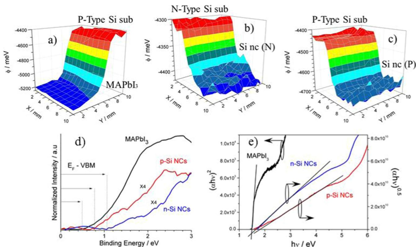
Fig. 5. Kelvin probe measurements to determine Fermi level of a) MAPbI<sub>3</sub>, b) n-type Si NCs and c) p-type Si NCs. d) XPS low binding energy scans where the onset of the signal relates to the energy separation  $E_F - \text{VBM}$  and e) Tauc plots to calculate the bandgap energy for MAPbI<sub>3</sub> and p- and n-type Si NCs.
