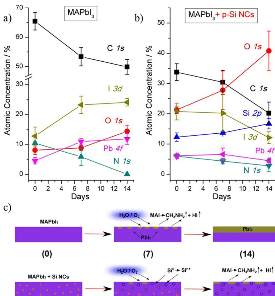
**Fig. 3.** Atomic concentration determined by XPS over time in atmosphere for a) MAPbI<sub>3</sub> films b) MAPbI<sub>3</sub> + p-Si NC films. c) schematic to show the typical MAPbI<sub>3</sub> surface degradation pathway (top) and the reduced degradation as a consequence of p- and n-Si NC inclusion (bottom).
