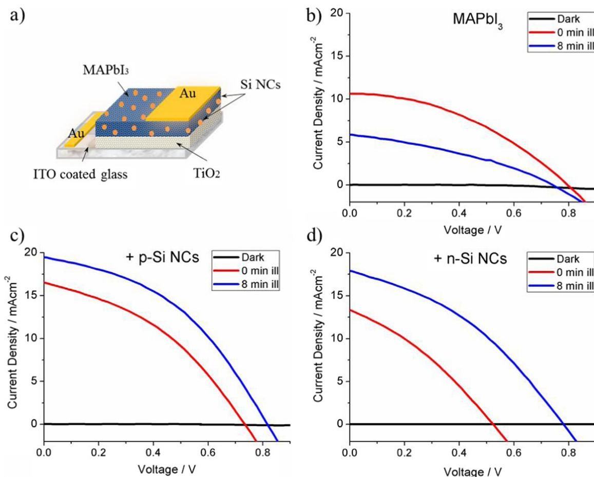
Fig. 8. a) MAPbI<sub>3</sub> based device structure b) current-voltage measurements in dark, at 0 min illumination and after 8 min illumination for MAPbI<sub>3</sub> only devices c) MAPbI<sub>3</sub> + p-Si NC and d) MAPbI<sub>3</sub> + n-Si NC solar devices.
