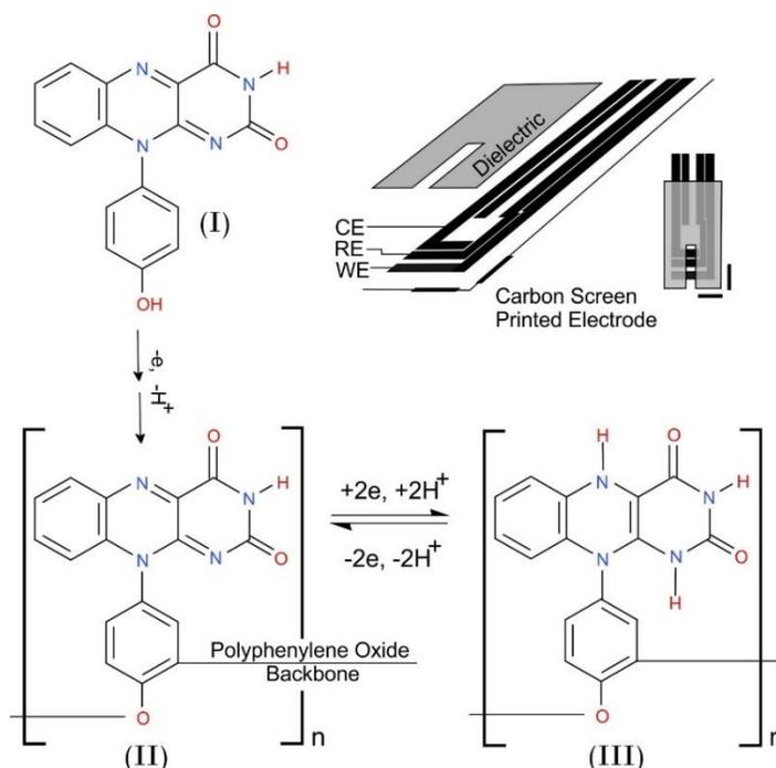
**Scheme 1.** Electro-oxidation of the flavin monomer leading to the production of the a polyphenylene oxide chain with pendant redox groups (**I**  $\rightarrow$  **II**) and the subsequent redox transitions of the flavin unit (**II**  $\rightarrow$  **III**  $\rightarrow$  **II**). Inset: Design of the screen printed sensor used throughout this work
