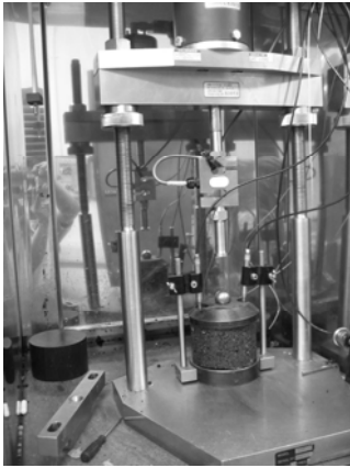
Figure 6. Repeated Load Axial Test (RLAT).
