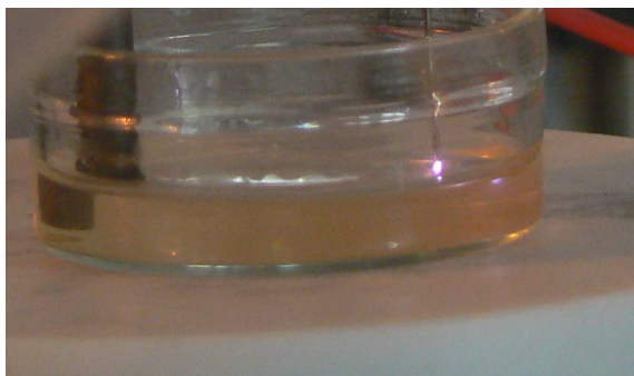
Fig. 2. Photograph of the AMP generated above the surface of the ethanol-SiNCs colloidal dispersion.
