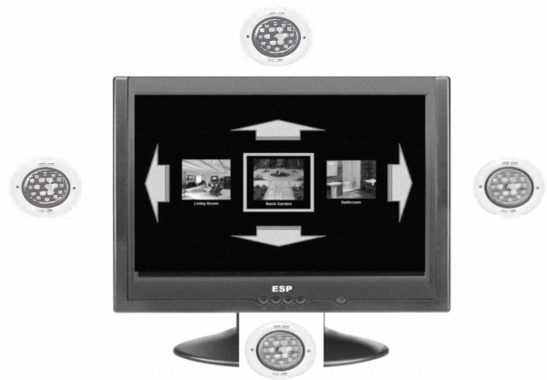
Figure 5. Four-Command Interface showing high level location menu by the IGUI. Four LED’s correspond with arrows to provide the command interface
