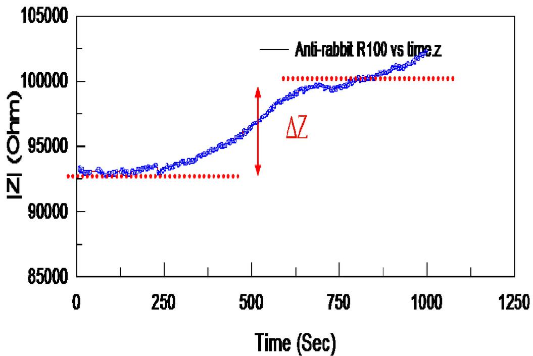
**Figure 4.** (a) Showing the Nyquist plot before and after adding secondary antibodies, (b) Showing the magnitude of impedance  $|Z|$  vs. time at a fixed frequency.
