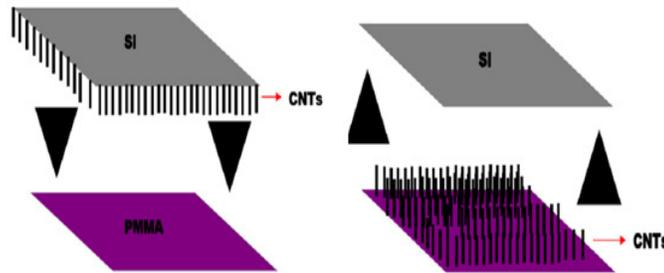
**Figure 1.** Schematic of hot embossing method using CNTs.
