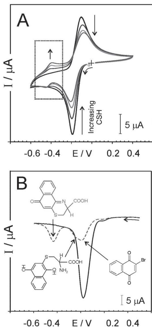
Fig. 3. Cyclic (A) and square-wave (B) voltammograms detailing the response of a glassy carbon electrode towards 0.5 mM NQBr (pH 7) in the presence of increasing cysteine, CSH, (55  $\mu$ M, dashed line). Scan Rate: 0.1 V/s.
