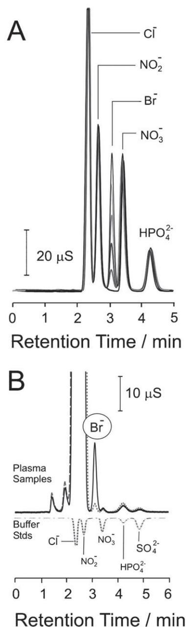
Fig. 4. Ion chromatograms detailing A) the release of bromide as a consequence of the reaction of NQBr with increasing concentrations of glutathione (250  $\mu$ M increments) and B) the response obtained to plasma before (dashed line) and after (solid line) reaction with NQBr.
