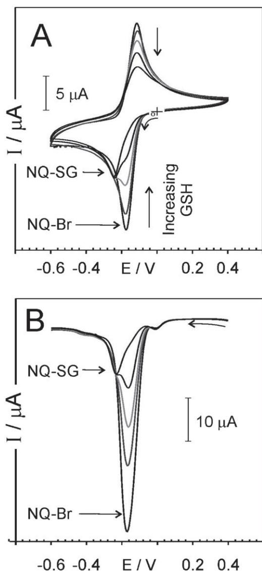
Fig. 1. Cyclic (A) and square-wave (B) voltammograms detailing the response of a glassy carbon electrode towards 0.5 mM NQBr (pH 7) in the presence of increasing glutathione, GSH, (55  $\mu$ M). Scan Rate: 0.1 V/s.
