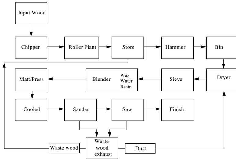
Figure 1. Basic flowsheet of the chipboard process plant.
