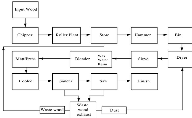
Figure 1. Basic flowsheet of the chipboard process plant.
