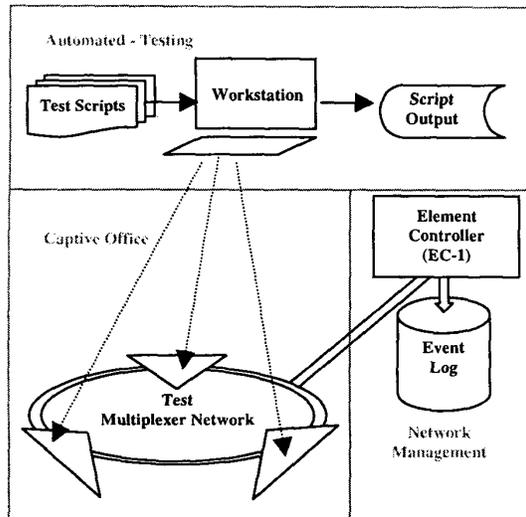
Figure 1: Verification Automated Testing of Network Elements (NE)
