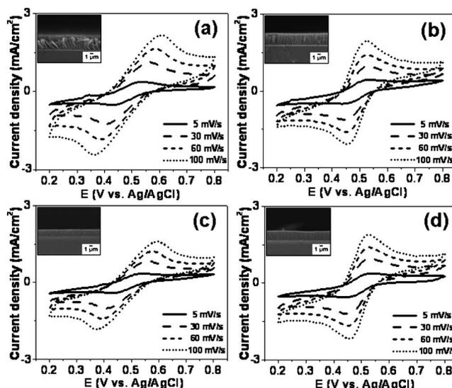
Fig. 1. Cyclic voltammograms of CN<sub>x</sub> NTs grown on Ti-(20 nm) buffered (a) *n*-type, (b) *n*<sup>+</sup>-type, (c) *p*-type, and (d) *p*<sup>+</sup>-type Si substrates. Insets are corresponding scanning electron microscope (SEM) cross-section views of CN<sub>x</sub> NTs.
