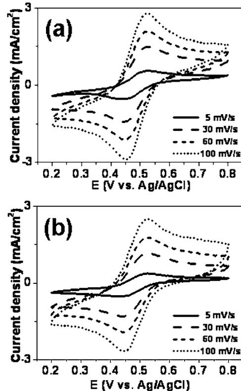
FIG. 3. Cyclic voltammograms of CN<sub>x</sub> NTs grown with a 200-nm-thick Ti buffer layer on (a) *n*-type and (b) *n*<sup>+</sup>-type Si substrates.
