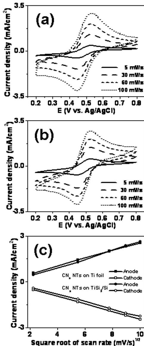
FIG. 5. Cyclic voltammograms of CN<sub>x</sub> NTs on (a) TiSi<sub>2</sub>/n-Si and (b) Ti foils. (c) The peak-current densities as a function of the square root of scan rate for both anode and cathode.
