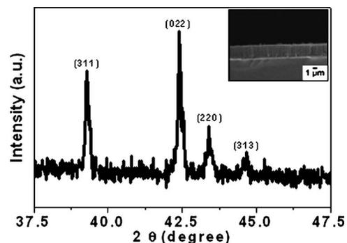
FIG. 4. XRD pattern shows TiSi<sub>2</sub> phase formation. The SEM image of CN<sub>x</sub> NTs on TiSi<sub>2</sub>/*n*-Si is shown in the inset.
