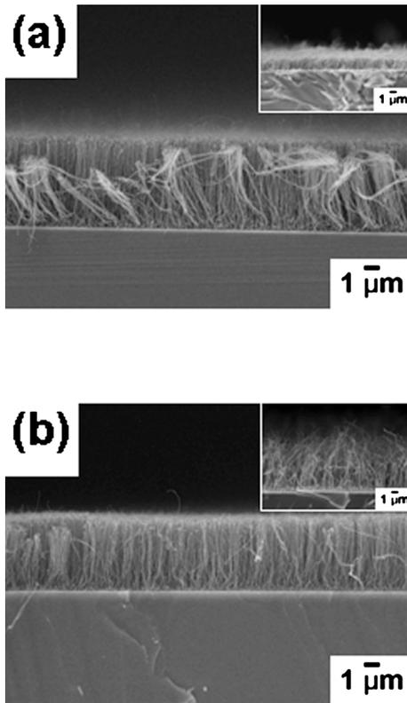
FIG. 2. Cross-section morphologies of SEM show CN<sub>x</sub> NTs grown with thermally oxidized catalyst on *n*-type Si with a Ti buffer-layer thicknesses of (a) 20 nm and (b) 200 nm. The insets are their counterparts without thermal oxidation.
