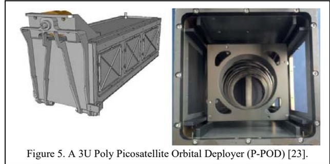
Figure 5. A 3U Poly Picosatellite Orbital Deployer (P-POD) [23].
